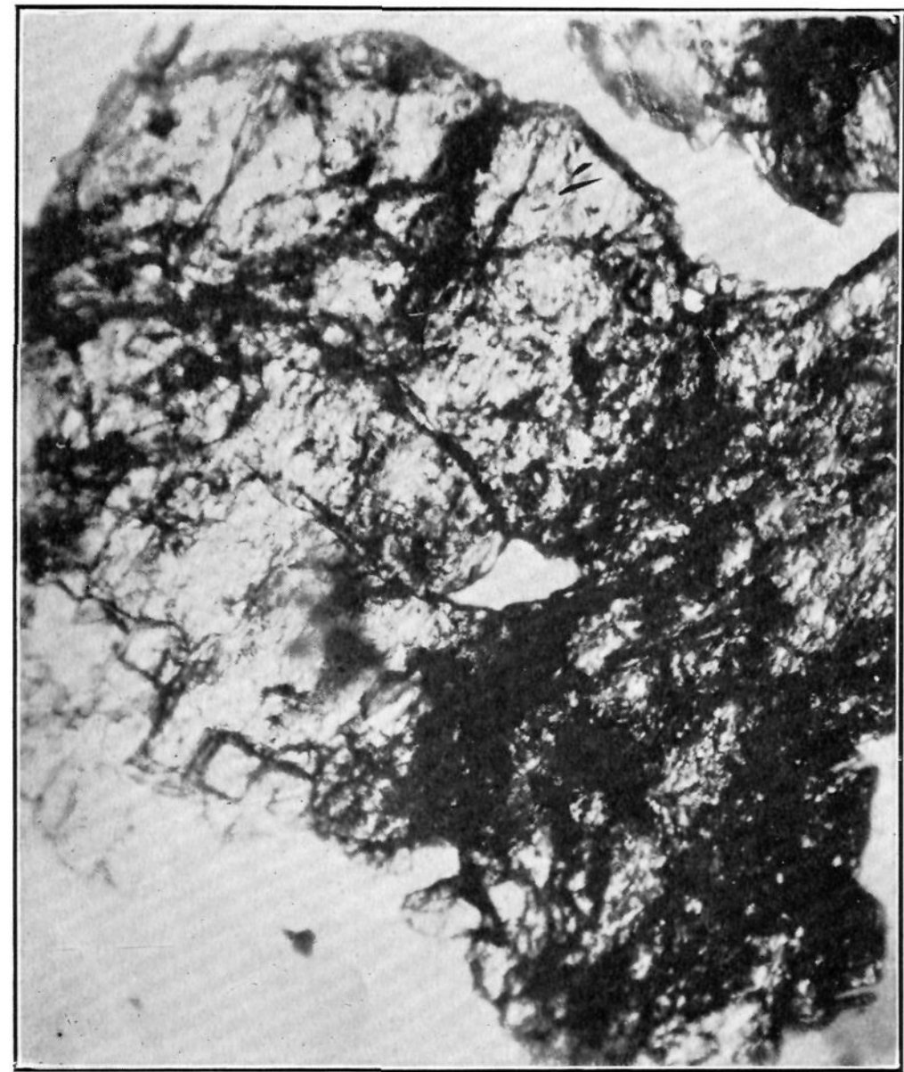
Fig. III.—Plate showing a section of monazite after treatment with hydrochloric acid. \times 70 .
